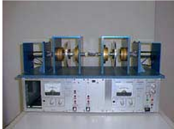
Figure 3. Swing Mass Model Apparatus
